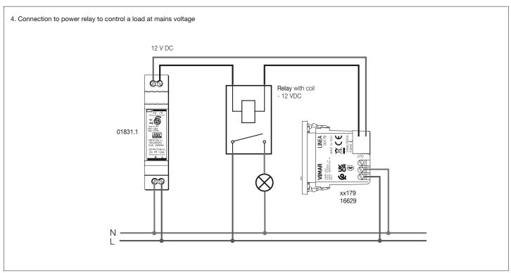
N.B. Graphic representation of the Linea series. Position of terminals, wiring and functions also identical for Eikon, Arké Idea and Plana.
