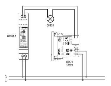
3. Connection to control switchboard or to device with potential-free inputs
