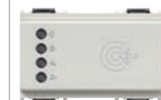
16927.B Transponder card reader for installation outside rooms, KNX standard, 2 NO 4 A 24 V~ relay outputs, 2 inputs, power supply 12-24 V~ 50/60 Hz and 12-24 Vdc (SELV), white - 3 modules. Supplied without transponder card. Depth: 36,5 mm
