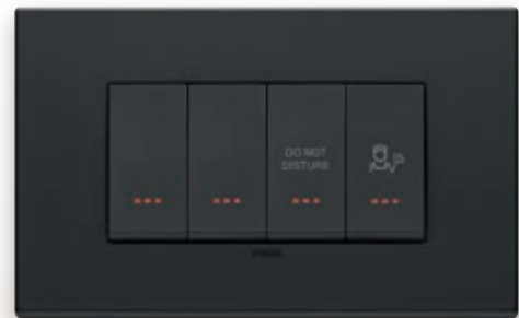
Switches for activating the two pilot lights "Do Not Disturb" and "Please Clean" for the special push button installed outside the room and connected 2-way switches to activate room lighting.
