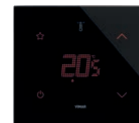
21514.S.76 Touch screen thermostat (heating and air conditioning), configurable STAR control, class I (contribution 1%) in ON/OFF mode, class IV (contribution 2%) in PID mode, can be interfaced with actuator 01466.1 to make a class V modulating room thermostat (contribution 3%), 1 input for sensor 20432, 19432 or 14432 or wired sensor 02965.1, 1 programmable digital input, RGB LED backlighting, black diamond - 2 modules. Depth: 30,2 mm
