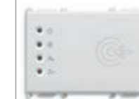
14457 Transponder card reader for installation outside rooms, KNX standard, 2 NO 4 A 24 V~ relay outputs, 2 inputs, power supply 12-24 V~ 50/60 Hz and 12-24 Vdc (SELV), white - 3 modules. Supplied without transponder card. Depth: 36 mm
