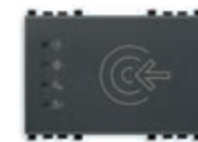
20457 Transponder card reader for installation outside rooms, KNX standard, 2 NO 4 A 24 V~ relay outputs, 2 inputs, power supply 12-24 V~ 50/60 Hz and 12-24 Vdc (SELV), grey - 3 modules. Supplied without transponder card. Depth: 37 mm
