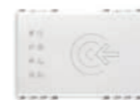
20457.B Transponder card reader for installation outside rooms, KNX standard, 2 NO 4 A 24 V~ relay outputs, 2 inputs, power supply 12-24 V~ 50/60 Hz and 12-24 Vdc (SELV), white - 3 modules. Supplied without transponder card. Depth: 37 mm
