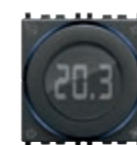
02971 Dial thermostat (heating and air conditioning), 2- and 4-pipe system management, 3-speed and proportional fan coil control, class I (contribution 1%) in ON/OFF mode, class IV (contribution 2%) in PID mode, can be interfaced with actuator 01466.1 to make a class V modulating room thermostat (contribution 3%), 1 input for sensor 20432, 19432, 14432 or 02965.1, white LED backlighting, grey - 2 modules. Depth: 28,5 mm
