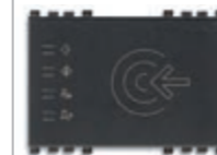
19457 Transponder card reader for installation outside rooms, KNX standard, 2 NO 4 A 24 V~ relay outputs, 2 inputs, power supply 12-24 V~ 50/60 Hz and 12-24 Vdc (SELV), grey - 3 modules. Supplied without transponder card. Depth: 37 mm
