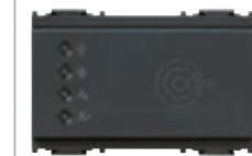
16927 Transponder card reader for installation outside rooms, KNX standard, 2 NO 4 A 24 V~ relay outputs, 2 inputs, power supply 12-24 V~ 50/60 Hz and 12-24 Vdc (SELV), grey - 3 modules. Supplied without transponder card. Depth: 36,5 mm
