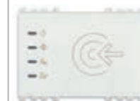
19457.B Transponder card reader for installation outside rooms, KNX standard, 2 NO 4 A 24 V~ relay outputs, 2 inputs, power supply 12-24 V~ 50/60 Hz and 12-24 Vdc (SELV), white - 3 modules. Supplied without transponder card. Depth: 37 mm
