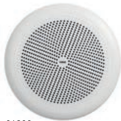
01906 IP55 passive speaker, 8 Ω 30 W, for hollow walls and false ceiling installation. Depth: 70 mm
