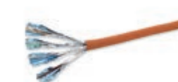
03086.E Cat. 6A S/FTP cable, shielded, 4-pair, 23 AWG, LSZH sheath, CPR Eca class, suitable for I category cables (U0 = 400 V), orange - 500 m
