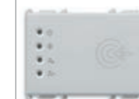
14457.SL Transponder card reader for installation outside rooms, KNX standard, 2 NO 4 A 24 V~ relay outputs, 2 inputs, power supply 12-24 V~ 50/60 Hz and 12-24 Vdc (SELV), Silver - 3 modules. Supplied without transponder card. Depth: 36 mm
