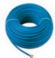
01840.E.B By-me system Bus cable for sound system, 2x0,50 mm 2 , with LSZH sheath, CPR Eca class, suitable for I category cables (U0 = 400 V), blue - 100 m
